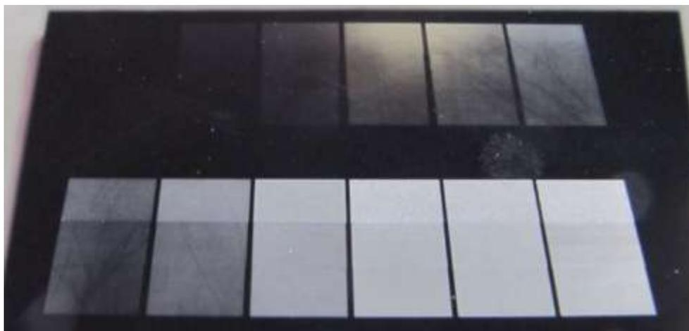
FIGURE 3 – PICTURE OF A GLASS-CERAMIC SAMPLE MARKED WITH UV-LASER
