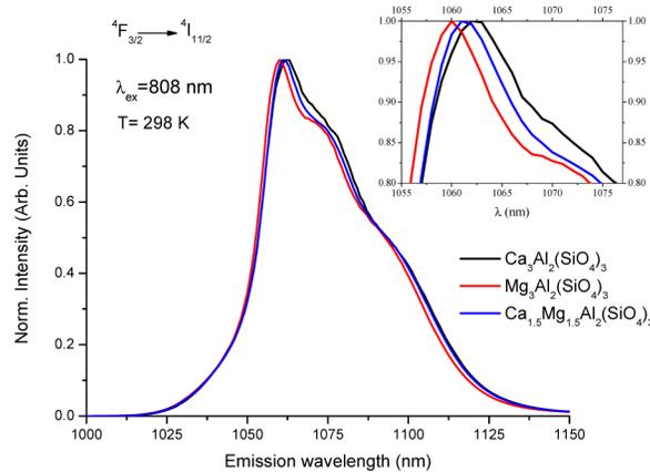
Fig. 3. Normalized fluorescence spectra of the <sup>4</sup>F<sub>3/2</sub>→<sup>4</sup>I<sub>11/2</sub> laser transition at room temperature measured by exciting the samples at 808 nm.
