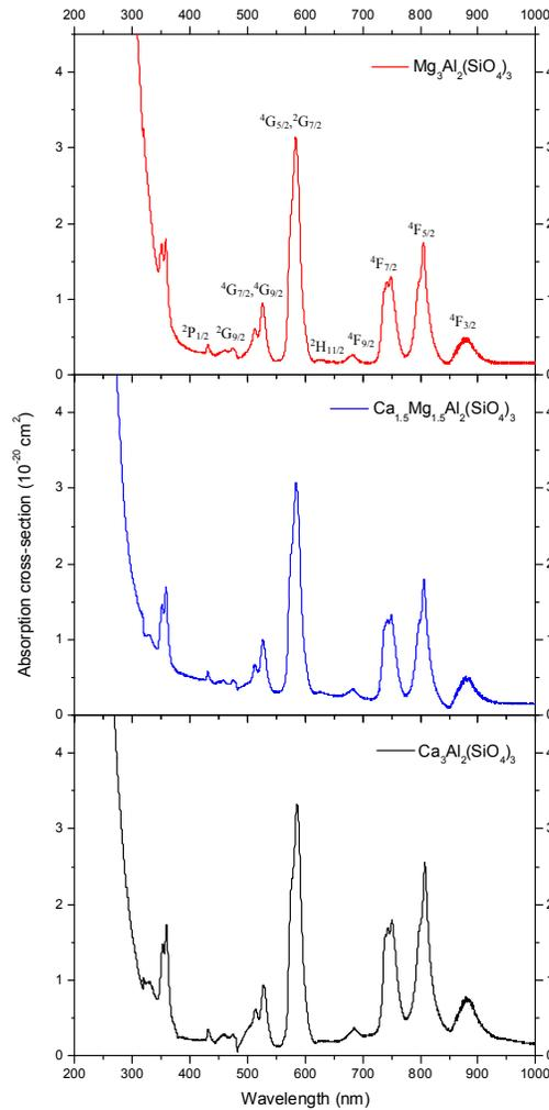
Fig. 1. Room temperature absorption cross-section spectra as a function of wavelength for  $\text{Ca}_3\text{Al}_2\text{Si}_3\text{O}_{12}$ ,  $\text{Ca}_{1.5}\text{Mg}_{1.5}\text{Al}_2\text{Si}_3\text{O}_{12}$  and  $\text{Mg}_3\text{Al}_2\text{Si}_3\text{O}_{12}$  glasses doped with Nd<sup>3+</sup> ions.
