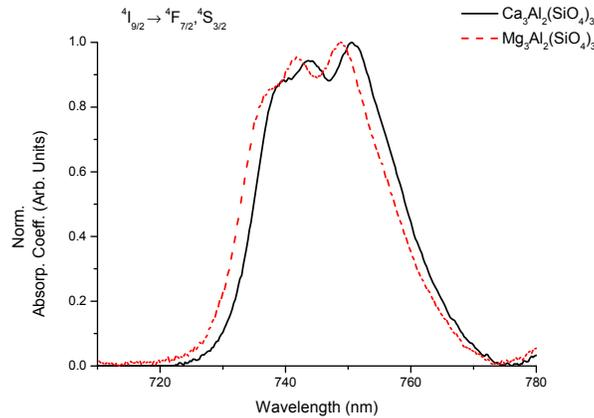
Fig. 2. Normalized <sup>4</sup>I<sub>9/2</sub>→<sup>4</sup>F<sub>7/2</sub>,<sup>4</sup>S<sub>3/2</sub> absorption transition for Ca<sub>3</sub>Al<sub>2</sub>Si<sub>3</sub>O<sub>12</sub>, and Mg<sub>3</sub>Al<sub>2</sub>Si<sub>3</sub>O<sub>12</sub> glasses doped with Nd<sup>3+</sup> ions.
